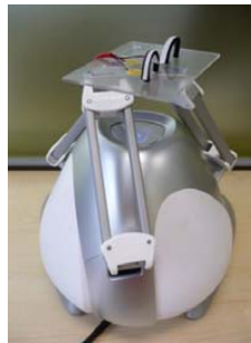
Fig. 2. Palpation device combining force feedback from a Novint Falcon and tactile feedback at the fingertips from piezoelectric materials. [18]
